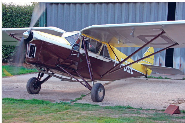
Maintaining as much original material as practicable, I-FOGL (2114), and her Gipsy III engine, was carefully dismantled and with meticulous care restored in the unique de Havilland style. On 13th September 2018, her engine was run for only the second time since 1936. (Tim Williams)
