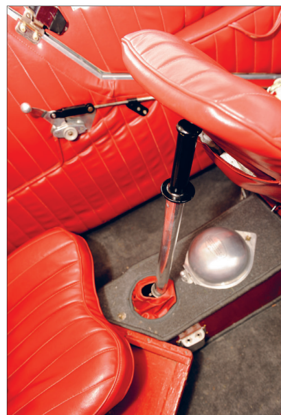
The Puss Moth could be fitted with a throttle control, stick and rudder pedals for operation by the occupant of the rear seat. The pedals were situated under the front seat and the rear control column could be easily disconnected and stowed alongside the control box at floor level. (Simon Clay)
