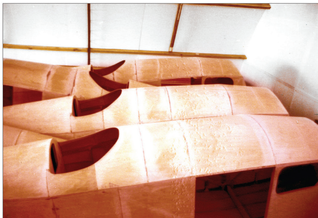
To satisfy the need for replacement fuselages for Fox Moth restoration projects in the mid-1970s, Myles Robertson and Stan Smith laid down five new fuselages and two additional 'kits' at Dairy Flat Airfield, Auckland. (Myles Robertson)
