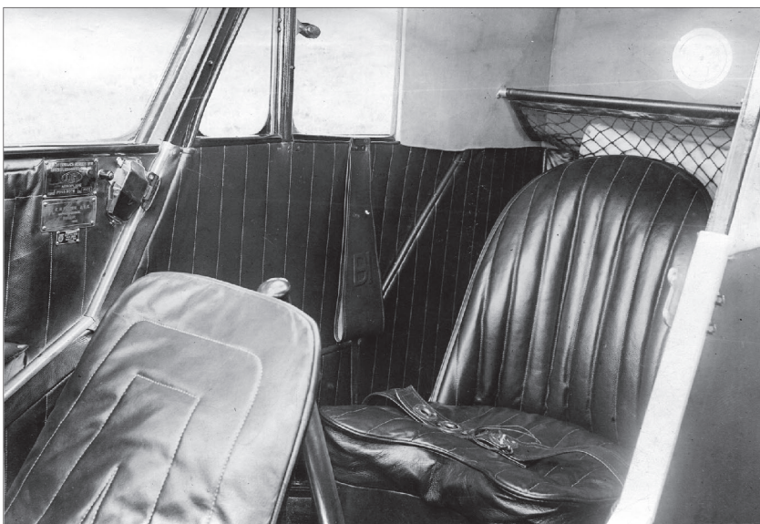
Royal Puss Moth G-ABBS (2020), was fitted with a single passenger seat in the rear of the cabin and a pilot's seat with a wide, flat, back support. Standard production aircraft, in which the pilot's seat had a rounded back, was criticised for being too narrow, partly the result of having to leave leg room for access to the rear passenger compartment.
