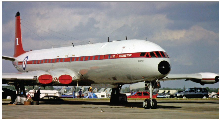
To meet Specification C.235 for a trials aircraft for navigation systems, Specification C.212 was used as the basis and Comet 4C XS235 Canopus was converted and fitted with a comprehensive suite of navigation aids and the equipment to record and analyse trials. Canopus survives at Bruntingthorpe in Leicestershire. (A-BDC)
