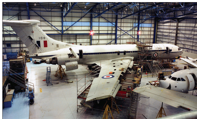
VC10 C.1 XV106 undergoing conversion to C.1K in the FRA hangar, Hurn. (via Author)
